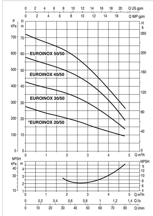
The performance curves are based on the kinematic viscosity values = 1 mm<sup>2</sup>/s and density equivalent to 1000 kg/m<sup>3</sup>. Curve tolerance according to ISO 9906.
