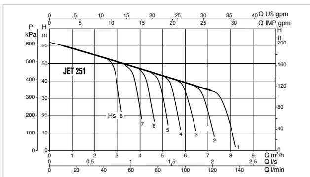
The performance curves are based on kinematic viscosity values = 1 mm<sup>2</sup>/s and density equivalent to 1000 kg/m<sup>3</sup>. Curve tolerance according to ISO 9906.
