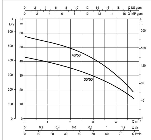
The performance curves are based on the kinematic viscosity values = 1 mm<sup>2</sup>/s and density equivalent to 1000 kg/m<sup>3</sup>. Curve tolerance according to ISO 9906.
