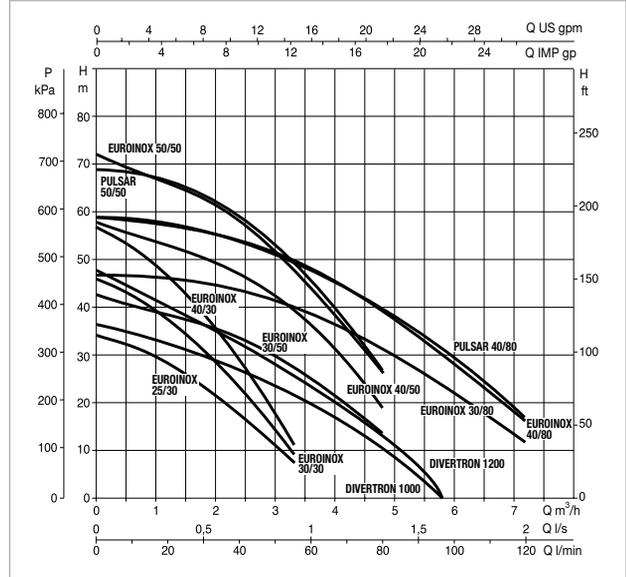
The performance curves are based on the kinematic viscosity values = 1 mm<sup>2</sup>/s and density equivalent to 1000 kg/m<sup>3</sup>. Curve tolerance according to ISO 9906.
