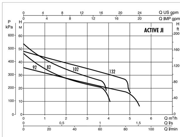
The performance curves are based on the kinematic viscosity values = 1 mm<sup>2</sup>/s and density equivalent to 1000 kg/m<sup>3</sup>. Curve tolerance according to ISO 9906.
