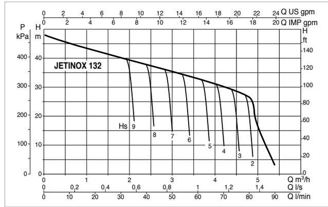
The performance curves are based on kinematic viscosity values = 1 mm<sup>2</sup>/s and density equivalent to 1000 kg/m<sup>3</sup>. Curve tolerance according to ISO 9906.
