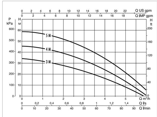
The performance curves are based on the kinematic viscosity values = 1 mm<sup>2</sup>/s and density equivalent to 1000 kg/m<sup>3</sup>. Curve tolerance according to ISO 9906.
